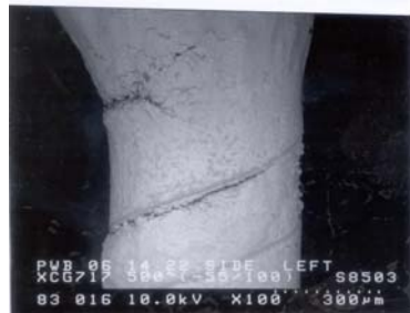
Figure 11 Optical photomicrographs of CCGA 717 I/O assembly (left) at 200 thermal cycles and their SEM Photomicrographs at 500 cycles. Some signs of damage at 500 cycles is apparent.
