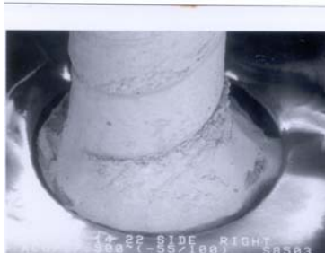
Figure 11 Optical photomicrographs of CCGA 717 I/O assembly (left) at 200 thermal cycles and their SEM Photomicrographs at 500 cycles. Some signs of damage at 500 cycles is apparent.
