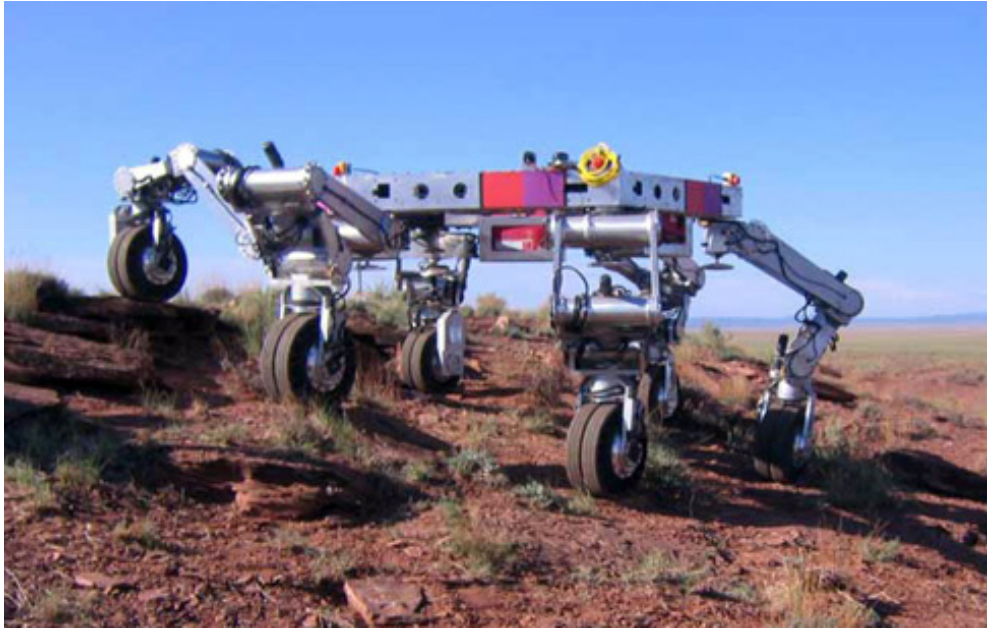
Figure 6: Testing of ATHLETE prototype being developed at Jet Propulsion Lab (JPL)
