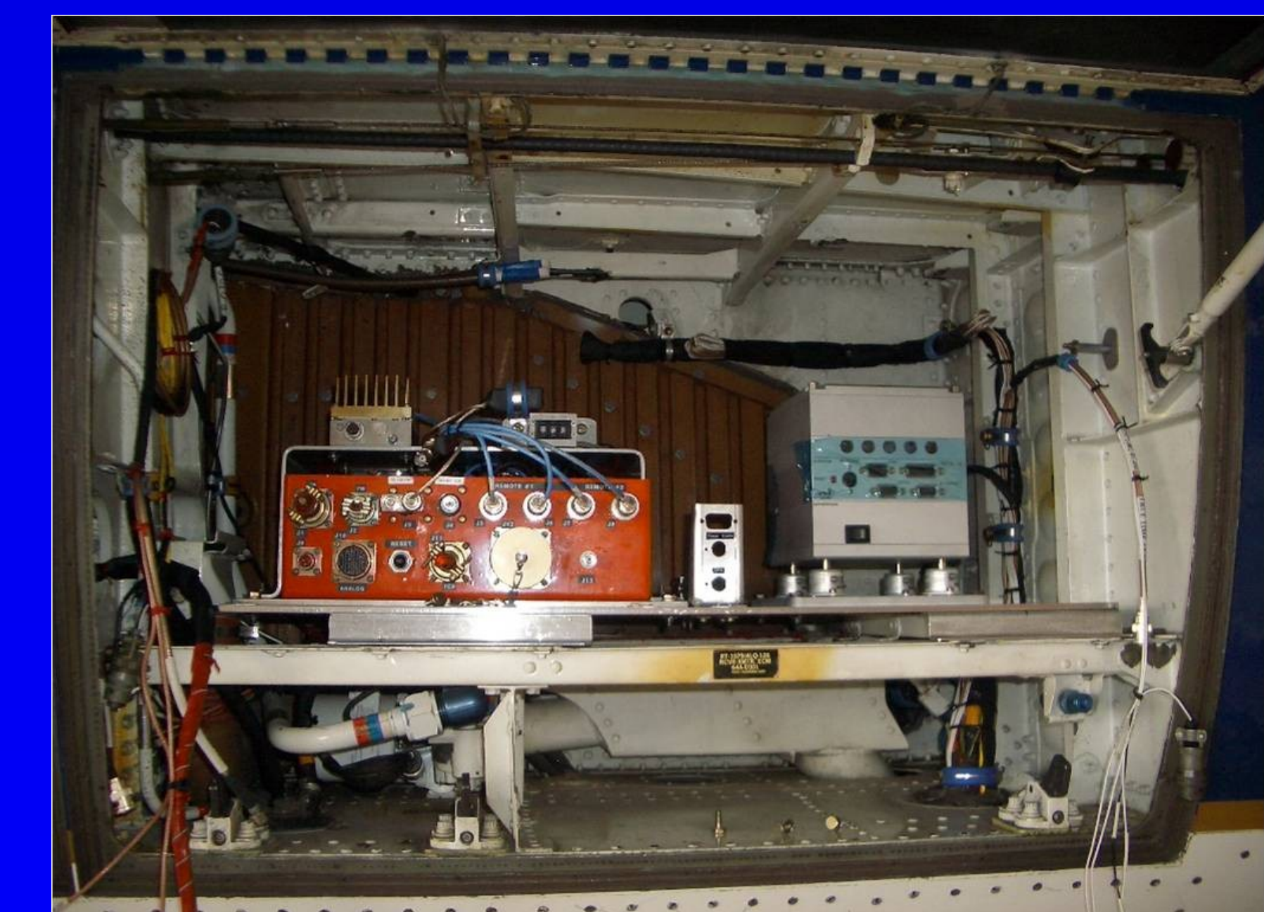
F-18/852 Avionics Bay with research instrumentation system
