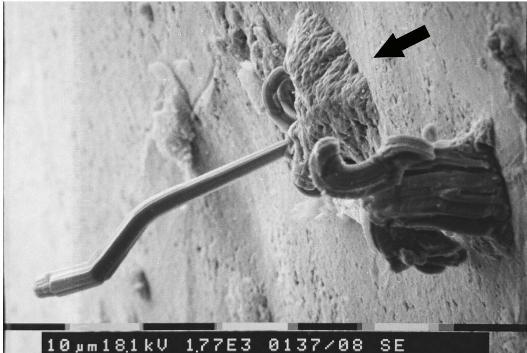
SEM image 5: A nodule with a hillock and a kinked filament.
