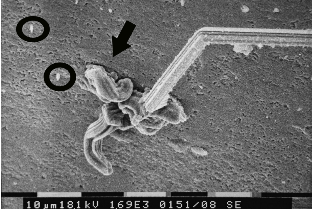
SEM image 3: A nodule flowing trough a surface crack, kinked filament whisker and “embryo whiskers”
