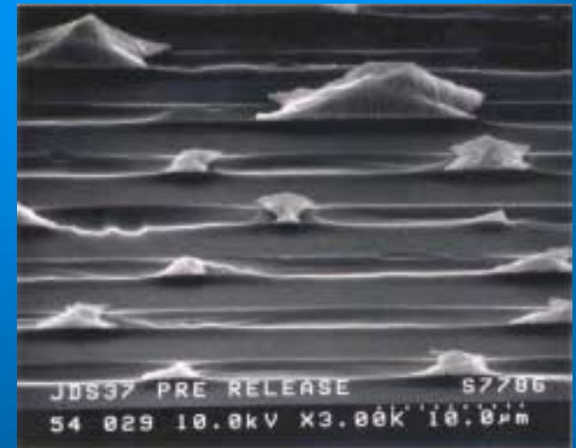
3000X SEM image of fractured unreleased cantilever beam array damaged during dicing.
