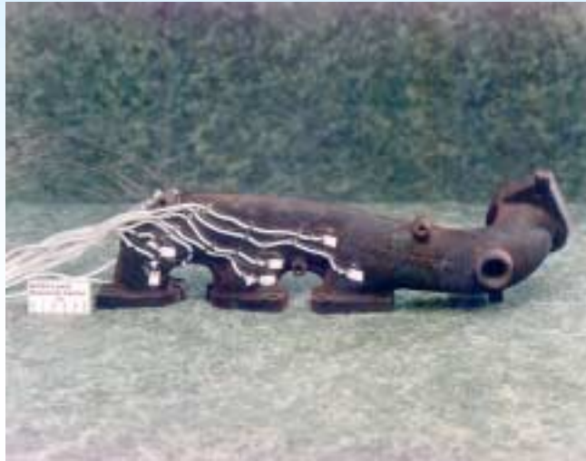
PdCr wire strain gauge applied on Ford Motor Co. exhaust manifold
