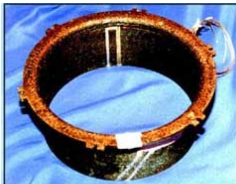
THIN FILM THERMOCOUPLES ON CERMIC MATRIX COMPOSITE HOOP
