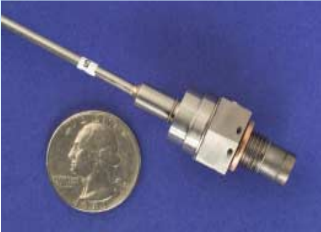
Above: 500 °C SiC pressure sensor
