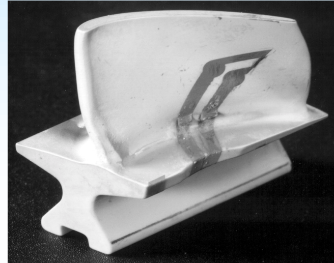
PdCr thin film gauge applied on Allied-Signal Engines ceramic turbine blade
