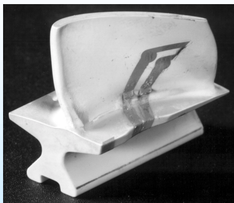
PdCr THIN FILM GAUGE APPLIED ON ALLIED-SIGNAL ENGINES CERAMIC TURBINE BLADE
