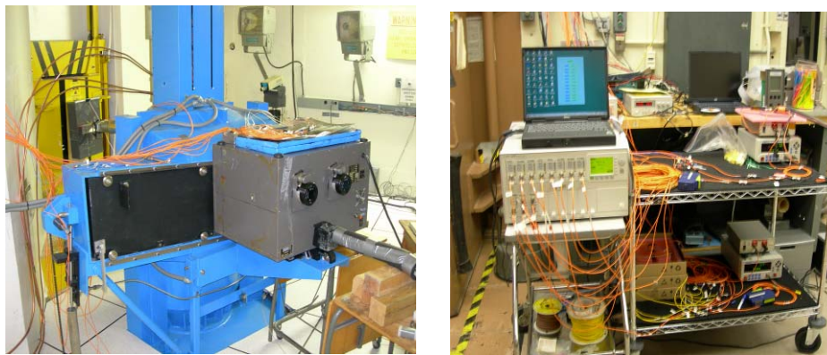
Figure 6 (a, b): Thermal Chamber Positioned in Front of Co60 Source and Data Gathering Setup
