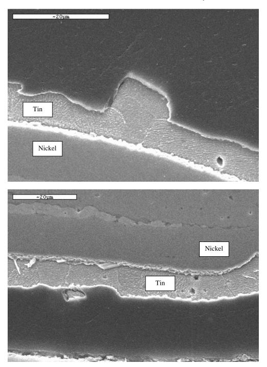
"Tin Etch" of the Cross Sectioned Ceramic Capacitor
