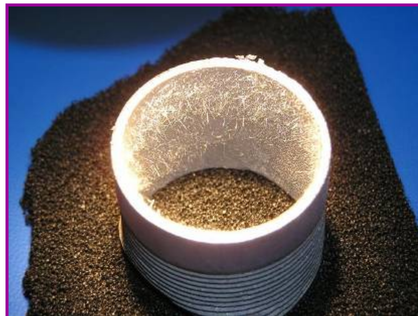
Zinc Whiskers on Hot Dip Galvanized Steel Pipe
