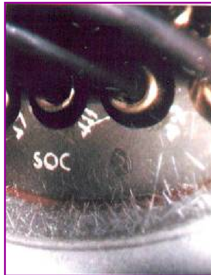
Cadmium-Plated Connector Shell Cadmium Whiskers
