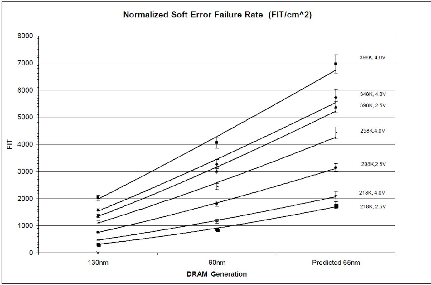
Figure 38. Normalized Soft Error Failure Rate for Scaled DRAM (FIT/cm<sup>2</sup>).
