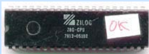
Zilog Z80 Processor circa 1978 8-bit processor
