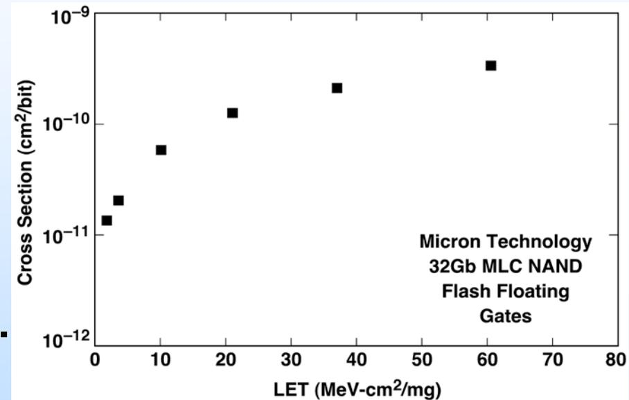
***–SEU cross-section for Micron Technology 32Gb MLC NAND flash memory, order of magnitude smaller than 8G MLC***
