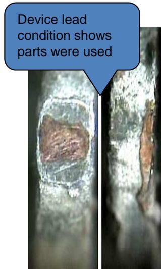
Device lead condition shows parts were used
