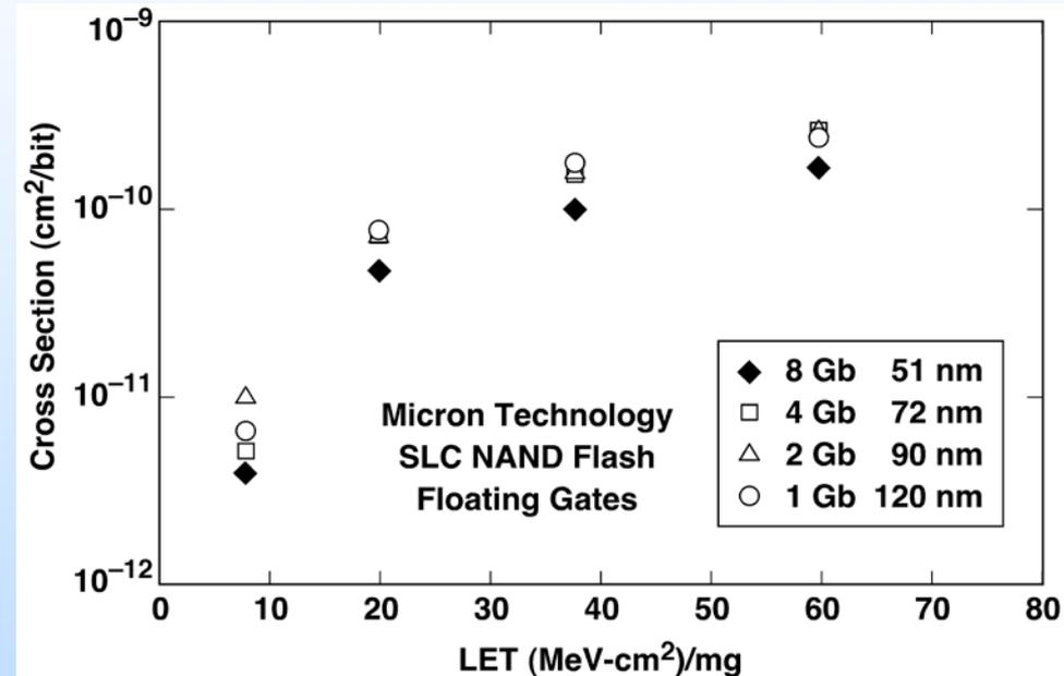
– *Measured SEU cross-sections for Micron Technology SLC NAND flash memories. Only minimal dependence on feature size.*
