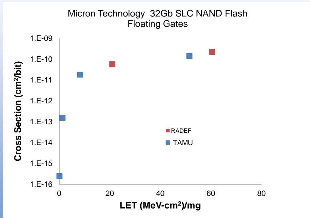
SEU cross-section for Micron 32Gb SLC NAND. Error bars are smaller than the plotting symbols
