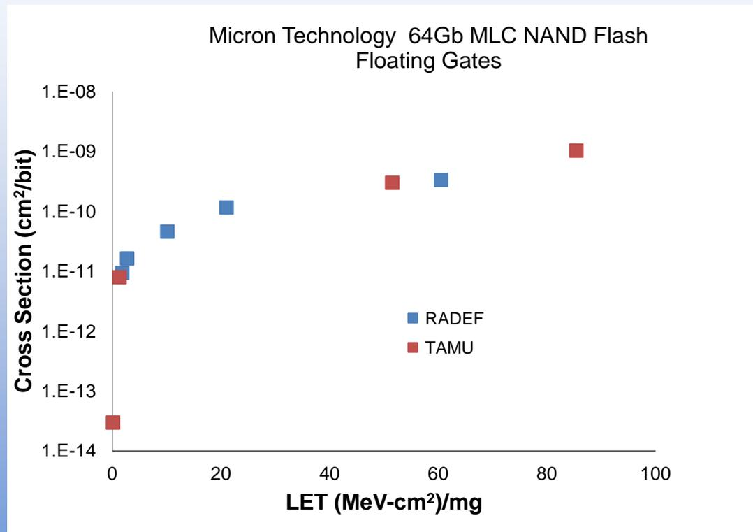
SEU cross-section for Micron Technology 64Gb MLC NAND flash memory. Error bars are smaller than the plotting symbols
