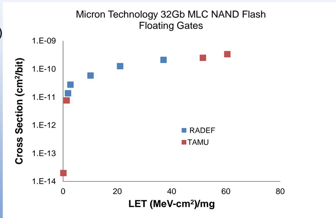
SEU cross-section for Micron 32Gb MLC NAND flash memory. Error bars are smaller than the plotting symbols
