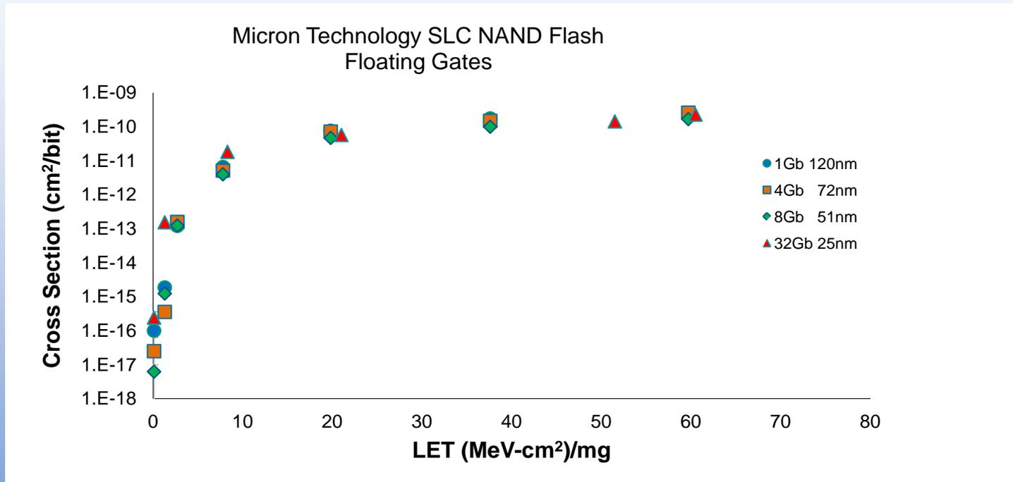
Scaling effect of FG SEU cross-sections for Micron SLC NAND flash memories. Error bars are smaller than the plotting symbols
