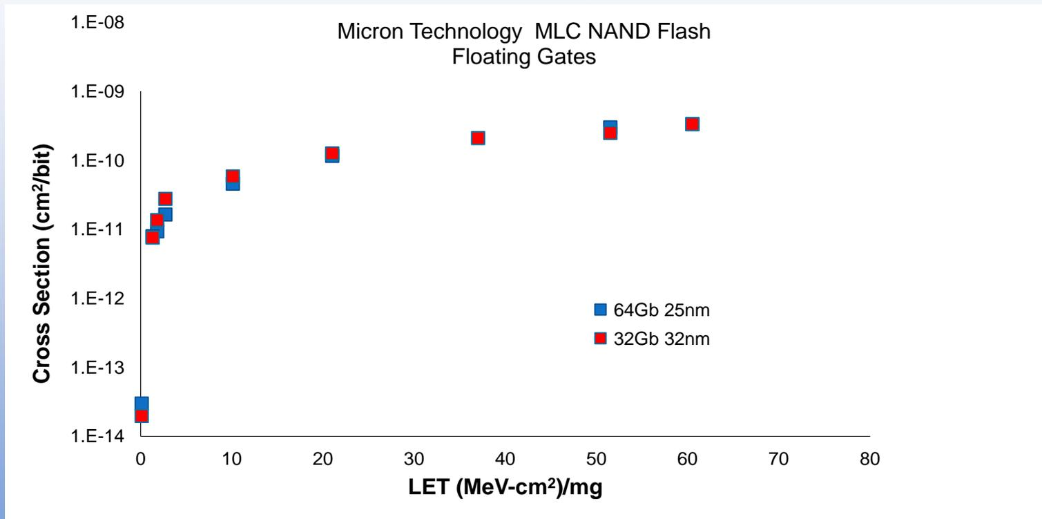
Scaling effect of FG SEU cross-section for Micron MLC NAND flash memories. Error bars are smaller than the plotting symbols
