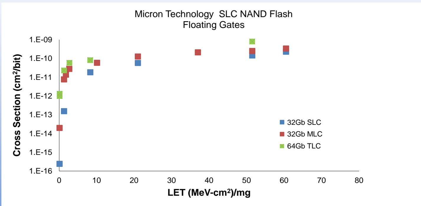
Comparison of SEU cross-section for Micron SLC, MLC and TLC NAND flash memories. Error bars are smaller than the plotting symbols.
