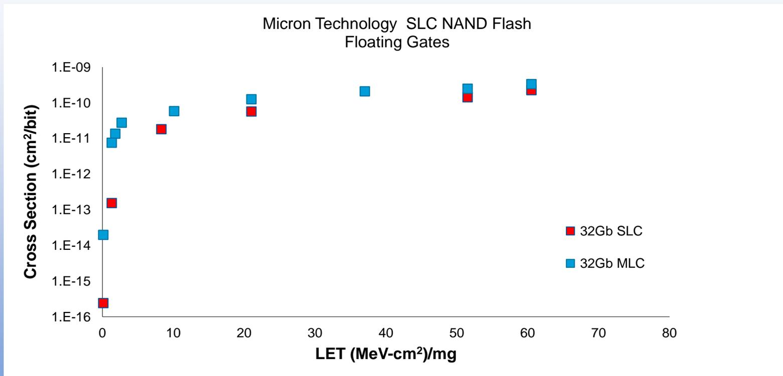
Comparison of SEU cross-section for Micron 32Gb SLC and MLC NAND flash memories. Error bars are smaller than the plotting symbols.
