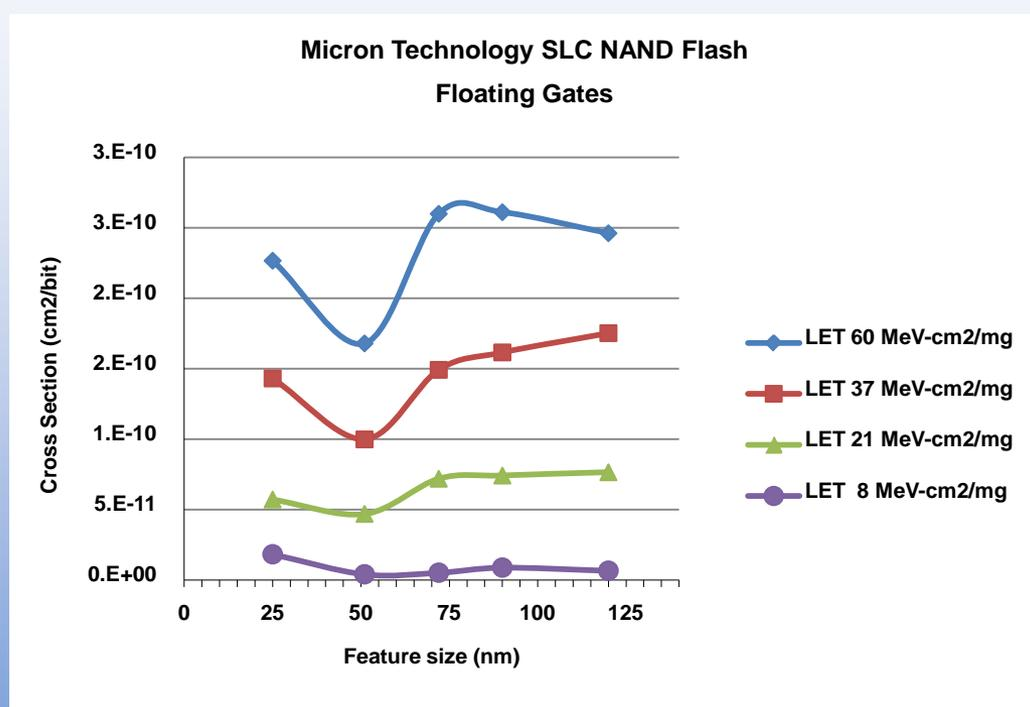
SEU cross-sections for Micron SLC NAND flash memories. Error bars are smaller than the plotting symbols
