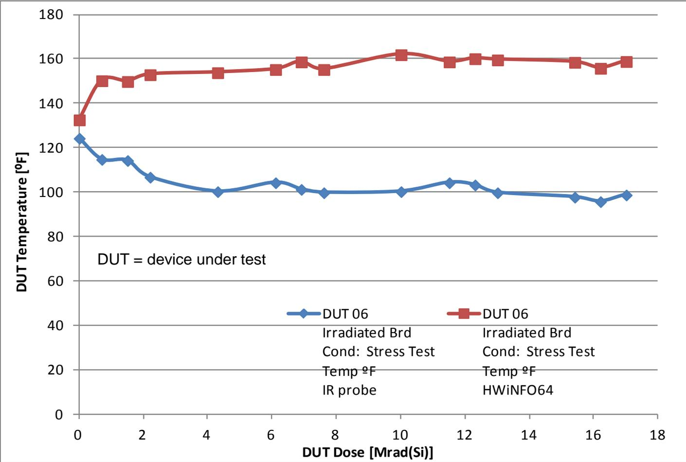
**Red** line indicates data points using processor’s temperature measurement circuit (diode?)
