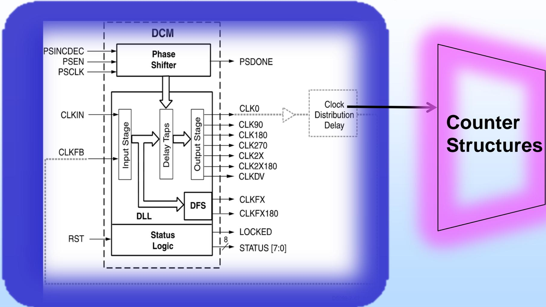
**We are testing DCM susceptibility by connecting the block to a design with a state space with feedback**
