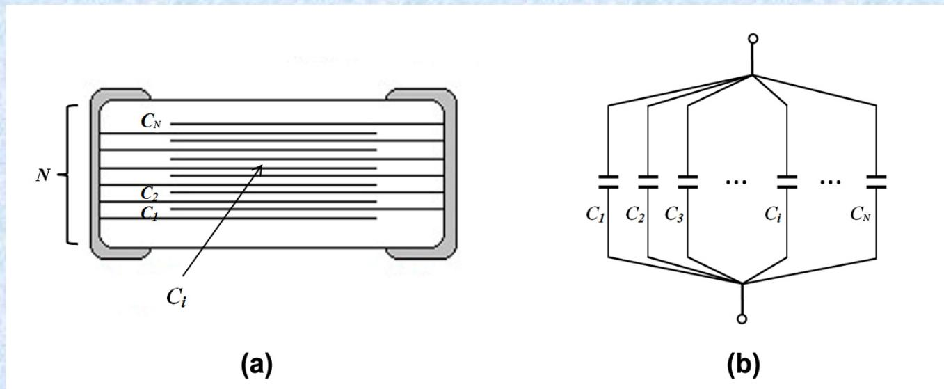
Total capacitance:  $C_t = C_1 + C_2 + C_3 \dots + C_i \dots + C_N = N \cdot C_i$
