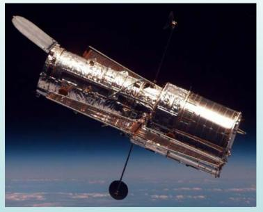
The Hubble Space Telescope (HST) is a 2.4-m (7.9-ft) aperture space telescope. It was carried into low Earth orbit by a Space Shuttle in 1990, and it remains in operation.
