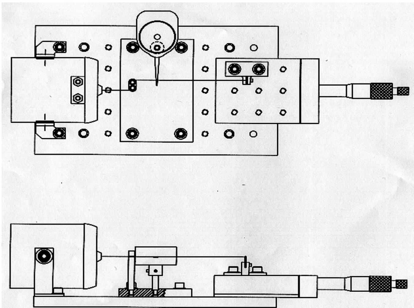
**Figure 6. Fatigue Fixture Incorporating the use of Mandrels.**
