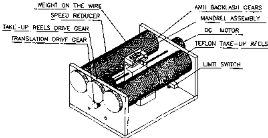
Fig 2 Fatigue machine
