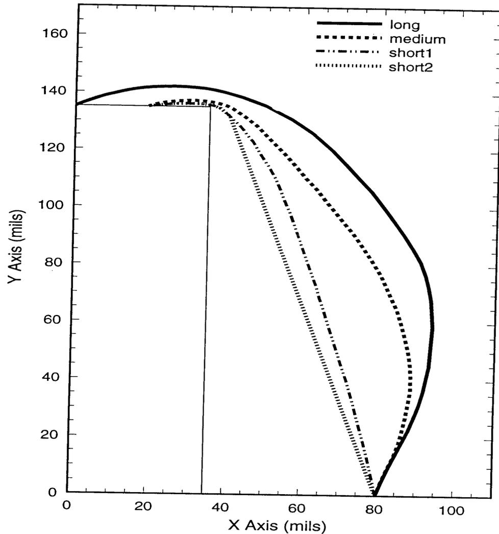
**Figure 1. Variation in the shape of bond wires observed in stacked memory modules.**
