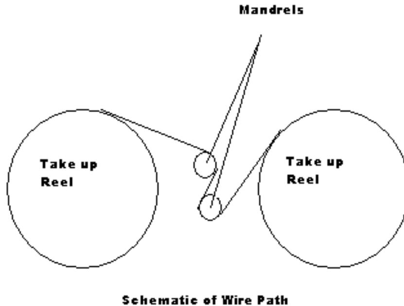
Figure 4. Wire path Schematic
