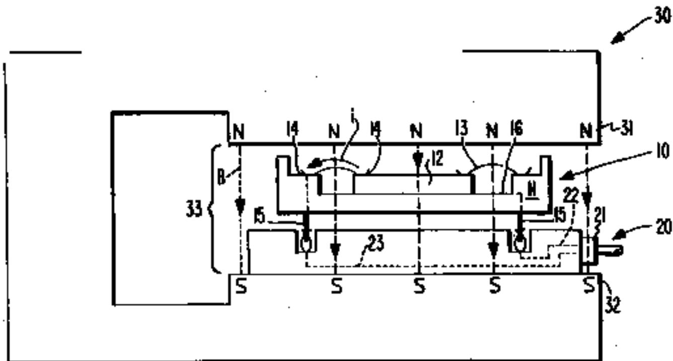
**Figure 3. Non-Destructive Bond Wire Tester Based on wire excitation**
