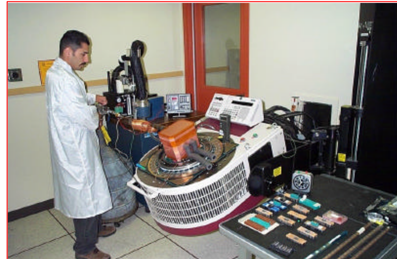
-125°C Cold ATE Digital Tester
