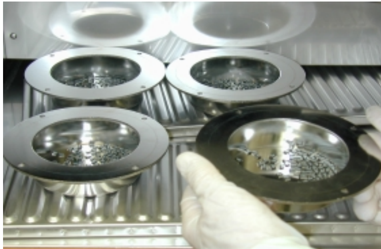
Figure 2: Loading of parts in the thermal chamber
