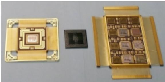
Figure 1. Various IC Packages: CQFP, PBGA, MCM
