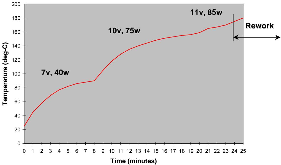
Figure 3. Integral Heater Thermal Transient, MCM Removal from PWB Rework Trial
