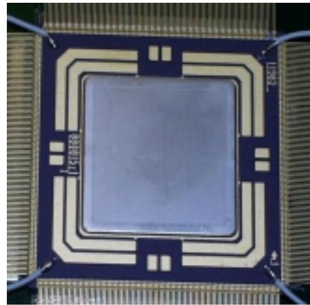
Figure 5. 352-Lead CQFP with Integral Heater
