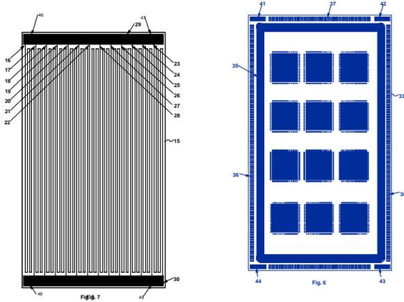
Figure 2. Integral Heater for 16-Layer MCM Package
