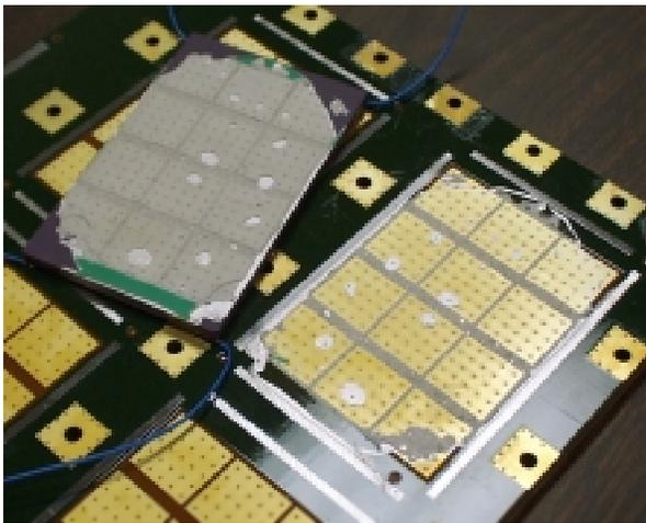
Figure 4. Successful Rework using Integral Heater
