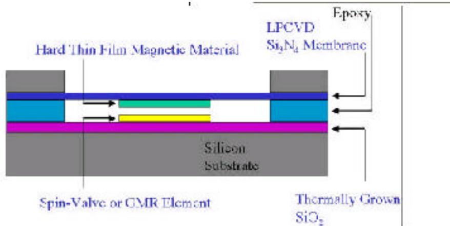
Figure 1. Schematic diagram of complete giant magnetoresistive (GMR) sensor device fabrication
