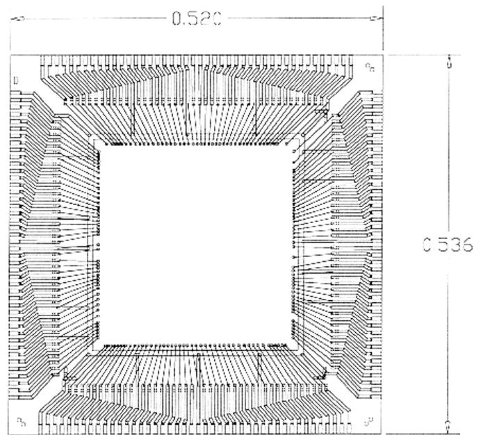
a) Snapstrate: trace width 6.5 mils, spaced 8.5 mils at the die end and 24 mils at the fan out end.
