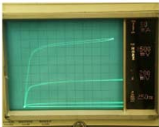
Figure 2a. Device #7 (7UD12G1T) npn characteristics before cycling.
