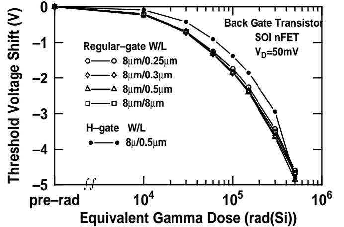
Fig. 7. Back-gate threshold voltage shift versus dose for regular-gate SOI nFET with different sizes and an H-gate SOI nFET.
