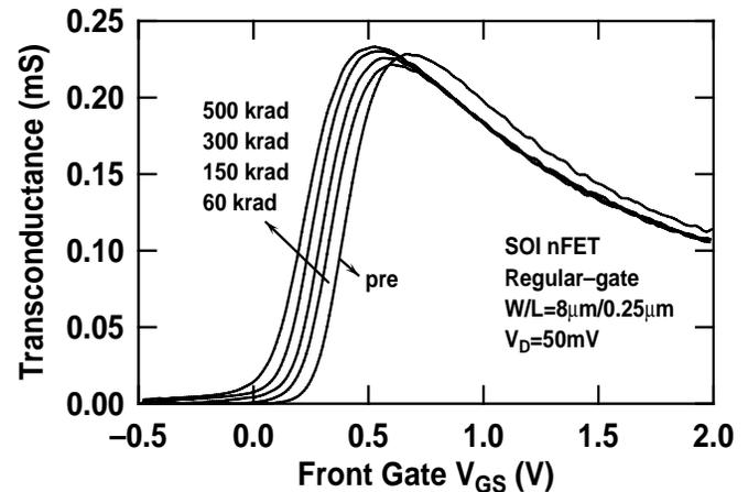
Fig. 12. Front-gate transconductance characteristics versus dose for a regular-gate SOI nFET.
