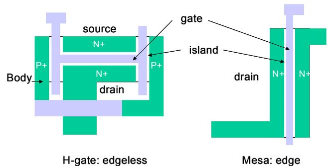
Fig. 1. The top-down views of the H-gate and regular-gate SOI MOSFETs configurations.
