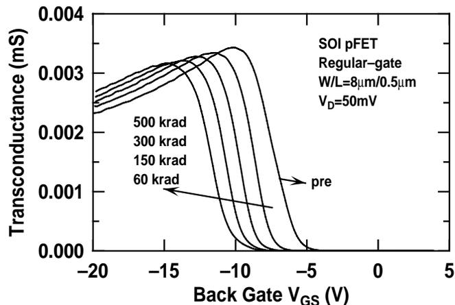
Fig. 16. Back-gate transconductance characteristics versus dose for a regular-gate SOI pFET.
