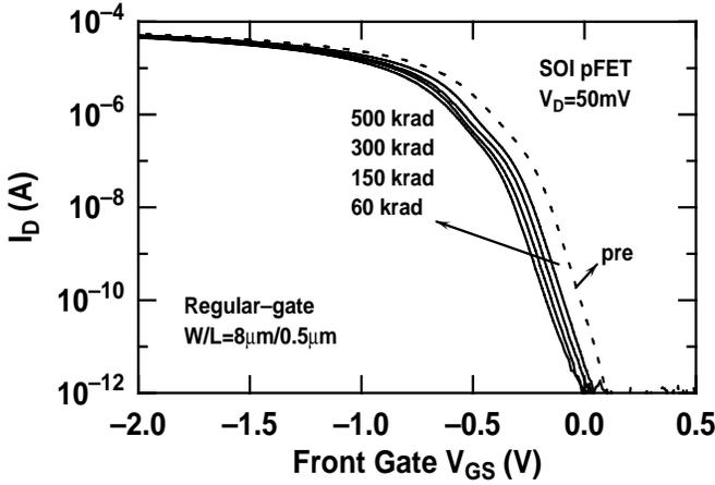
Fig. 5. Front-gate subthreshold characteristics versus dose for a regular-gate SOI pFET.
