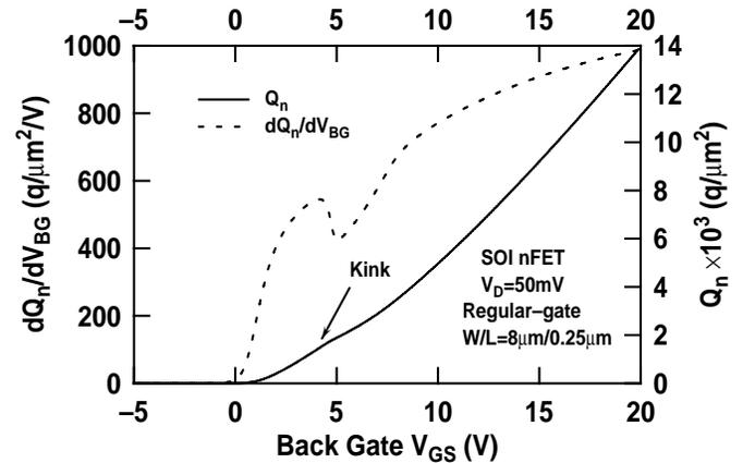
Fig. 15. The electron charge density at the Si/buried oxide interface versus the back-gate voltage, and the differential of the electron charge density with respect to back-gate voltage versus the back-gate voltage.
