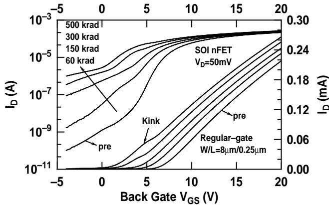
Fig. 8. Back-gate subthreshold and linear characteristics versus dose for a regular-gate SOI nFET.
