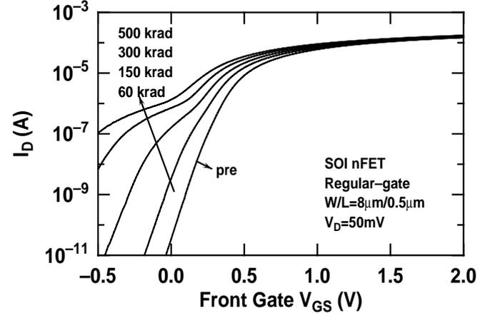
Fig. 3. Front-gate subthreshold characteristics versus dose for a regular-gate SOI nFET.
