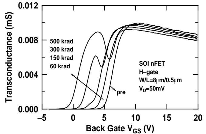
Fig. 11. Back-gate transconductance characteristics versus dose for an H-gate SOI nFET.
