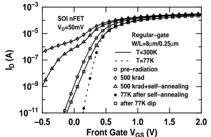
Fig. 17. Front-gate subthreshold characteristics versus dose and temperature for a regular-gate SOI nFET.
