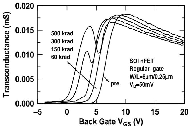
Fig. 10. Back-gate transconductance characteristics versus dose for a regular-gate SOI nFET.
