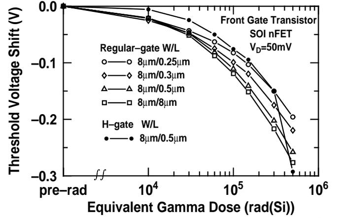
Fig. 6. Front-gate threshold voltage shift versus dose for regular-gate SOI nFETs with different sizes and an H-gate SOI nFET comparison.
