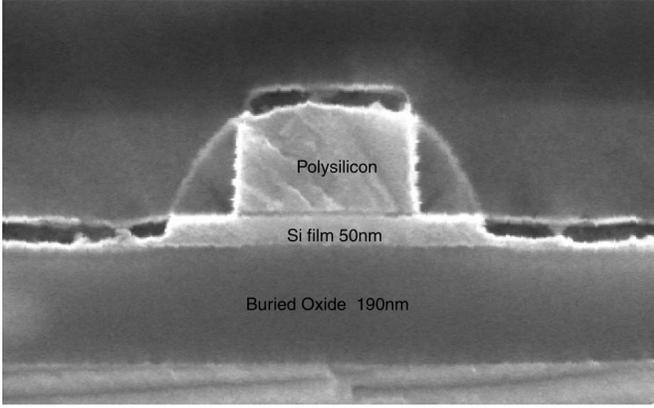
Fig. 2. SEM cross-section of a regular-gate SOI nFET.
