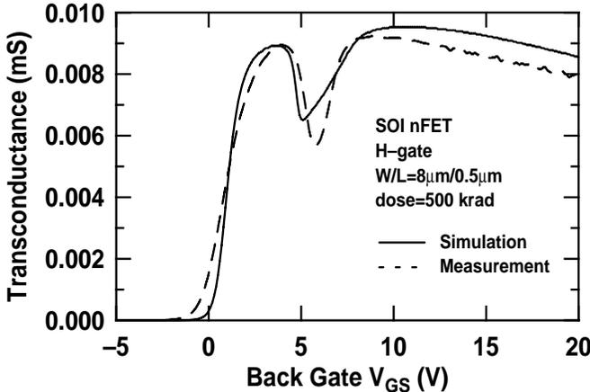
Fig. 14. Comparison of simulated and measured back-gate transconductance versus back-gate voltage.
