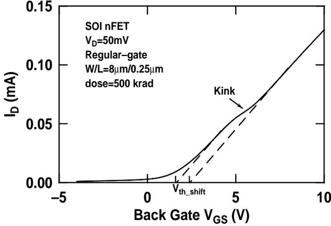
Fig. 13. Back-gate threshold voltage shift for a regular-gate nFET after 500krad irradiation.
