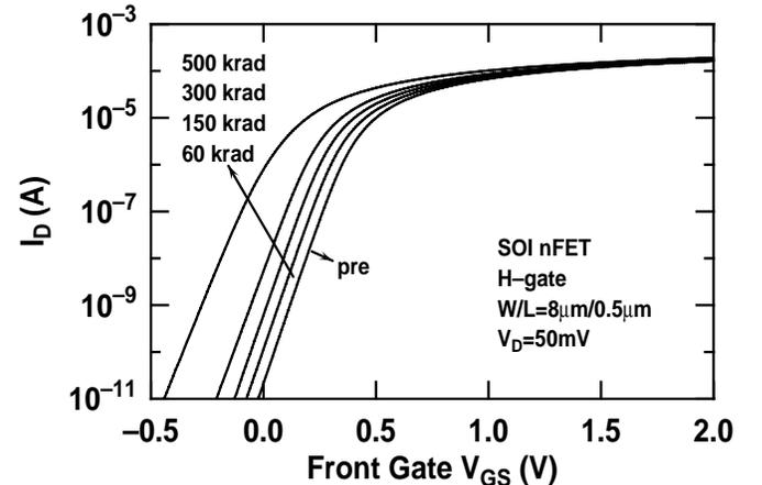
Fig. 4. Front-gate subthreshold characteristics versus dose for an H-gate SOI nFET.
