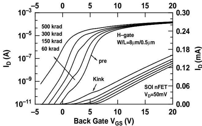
Fig. 9. Back-gate subthreshold and linear characteristics versus dose for an H-gate SOI nFET.
