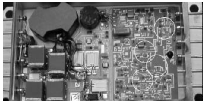
Figure 5. Photograph of the LCM-120 device with the four sensitive components circled in yellow.
