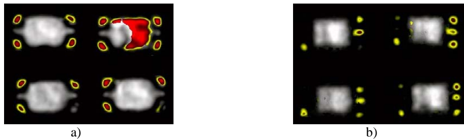
Fig. 1. Example of delaminations at the finger-tips on the top (a) and the bottom (b) of the SOT-23-5 packages after HAST.
