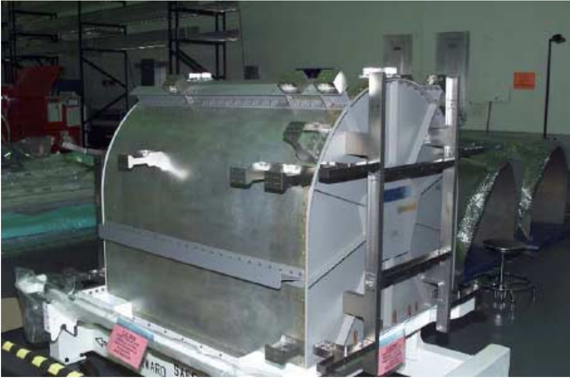
Figure 2: One of the four high pressure gas tanks which will be mounted on the exterior of the Joint Airlock to support EVA operations.
