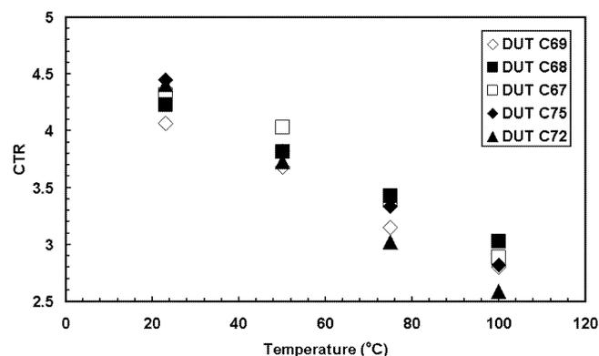
Fig. 14. Temperature effects on CTR for an Isolink 4N49 optocoupler.
