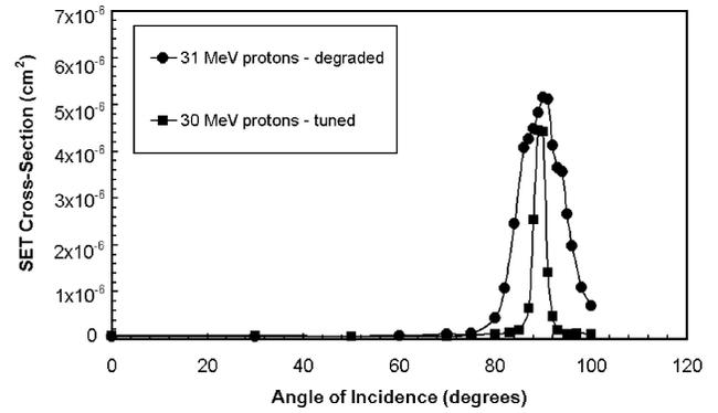
Fig. 3. Comparison of SET cross section measurement for degraded and tuned 30 MeV proton beam on the Agilent HCPL5231 optocoupler.
