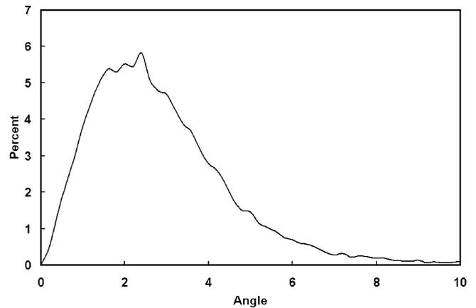
Fig. 4. TRIM calculation for trajectory of a 63 MeV proton after passing through 1.2 cm of Al. The exiting energy was  $\sim 30$  MeV.
