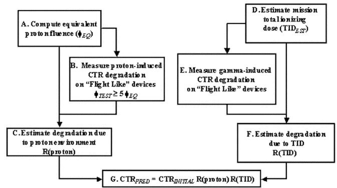
Fig. 10. Process for estimating CTR degradation.
