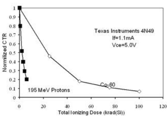
Fig. 9. Gamma and 195 MeV proton irradiations of Texas Instruments 4N49 [7].
