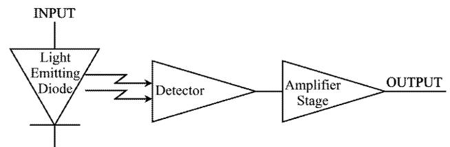
Fig. 1. Typical optocoupler design. The receiver side contains a detector and possibly a simple amplification stage [7].
