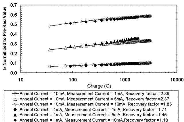
Fig. 13. Injection current annealing effect on collector current at two forward currents for three application currents. The data is normalized to the pre-irradiation collector currents.
