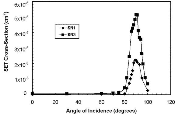
Fig. 5. Example of part to part dispersion observed during proton SET characterization of the Agilent HCPL5231.
