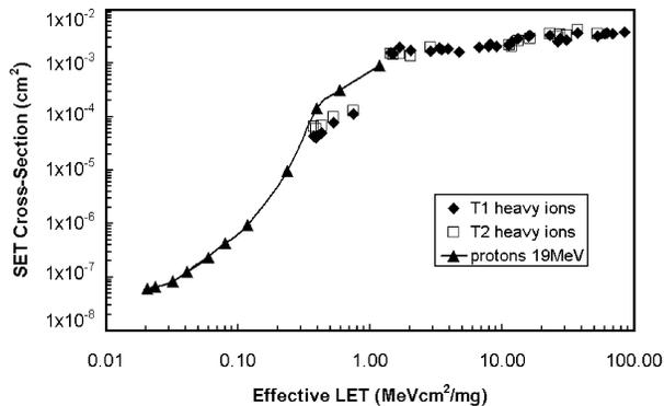
Fig. 7. Transient cross section for heavy ion and proton effective LET.
