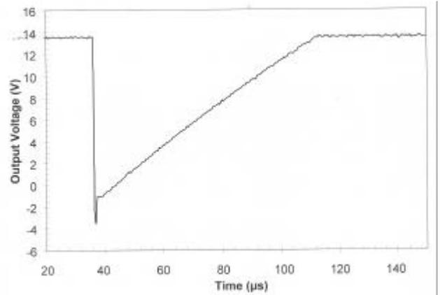
Fig. 12. LM124, voltage comparator application, typical large negative going transient, Transistor Q12 irradiated with a 64 pJ laser beam, Vcc = +/- 15V, V+ = 0.05V, V- = 0V.
