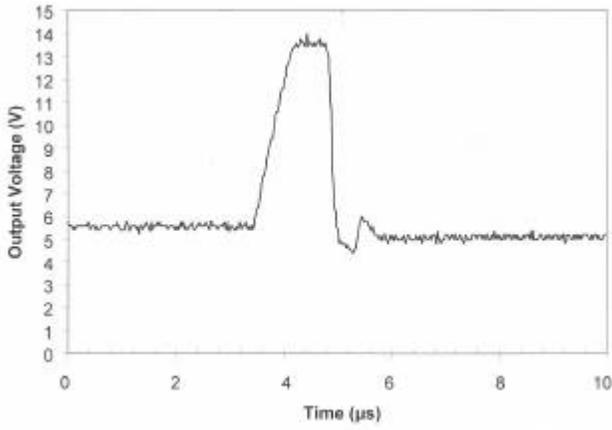
Fig. 8. LM124, Non inverting gain x101 application, typical large bipolar transient at low LET, LET = 2.86 MeVcm2/mg, Vcc = +/- 15V, V+ = 0.05V.
