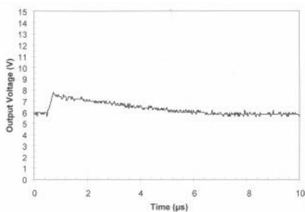
Fig. 10. LM124, Non-inverting gain x11 application, typical long duration transient observed at high LET, LET = 30 MeVcm2/mg, Vcc = +/- 15V, V+ = 0.5V.
