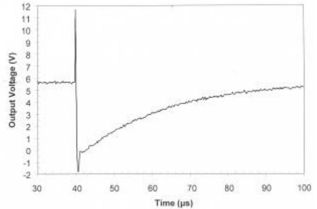
Fig. 13. LM124 Non-inverting gain application x101, typical bipolar transient, Transistors Q5/Q6 irradiated with a 214 pJ laser beam, Vcc = +/- 15V, V+ = 0.05V.
