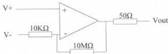
Fig. 1. LM124 Voltage comparator application circuit schematics.
