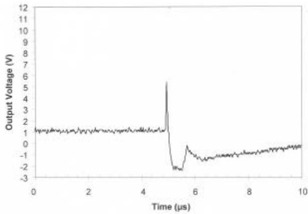
Fig. 9. LM124, Non-inverting gain x11 application, large bipolar transient at high LET with a small positive going component, LET = 30 MeVcm2/mg, Vcc = +/- 15V, V+ = 0.1V.
