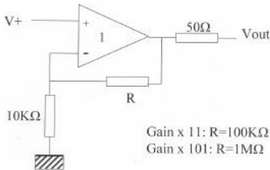
Fig. 2. LM124 Non inverting gain application circuit schematics.
