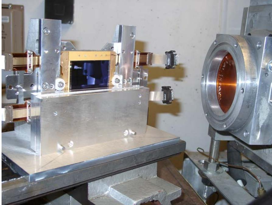
Figure 1. Test fixture for the BAE CCD486 proton test.
