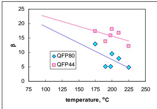
Figure 5. Temperature dependence of the shape parameter  $\beta$ .
