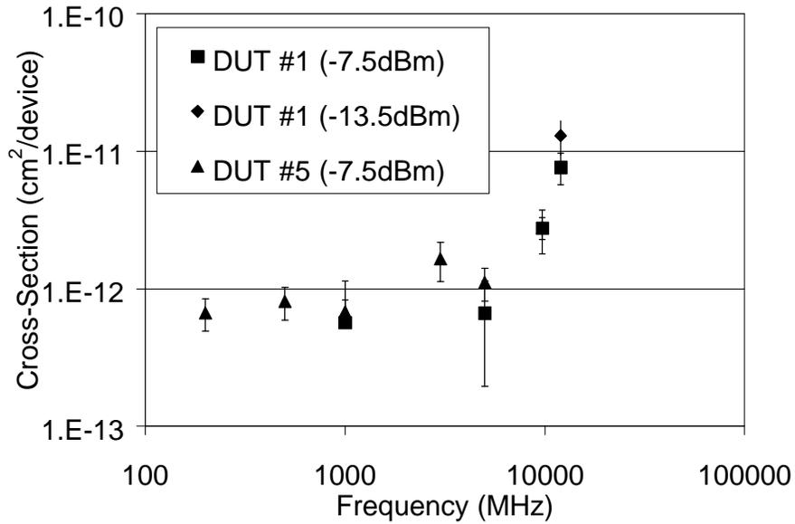
Figure 4. Synchronization error cross-section for the PRN when exposed to 200 MeV protons
