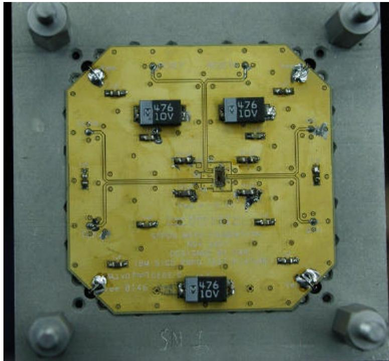
Figure 1. Picture of the high performance dielectric printed circuit board. The PRN is mounted near the center of the board. The input and output SMA and SMB connectors are mounted on the far side. (The plastic cover has been removed in this picture).
