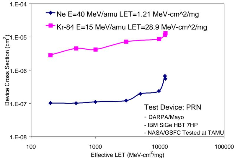
Figure 4. Synchronization error cross-section for the PRN when exposed to two heavy ion species
