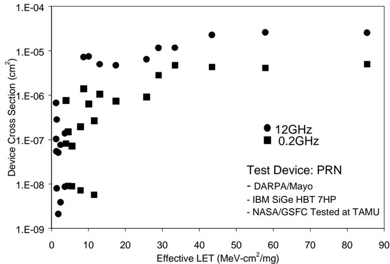
Figure 5. Heavy-ion results for synchronization errors on the PRN for various effective LETs
