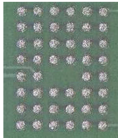
Figure 2 Solder paste on pads
