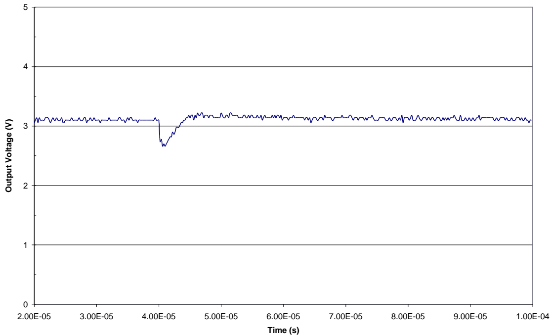
Figure 27: LM124, Non Inverting Gain1 application, location 2, typical pulse for a laser energy of 214 pJ.
