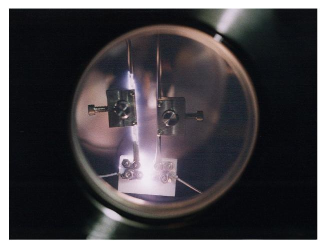
• First demonstration of a sustained tin plasma, generated by a single Tin-Whisker
