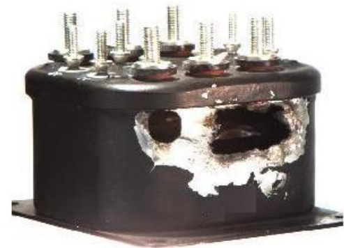
Relay destroyed by a metal vapor arcing event. Courtesy of Northrup Grumman
