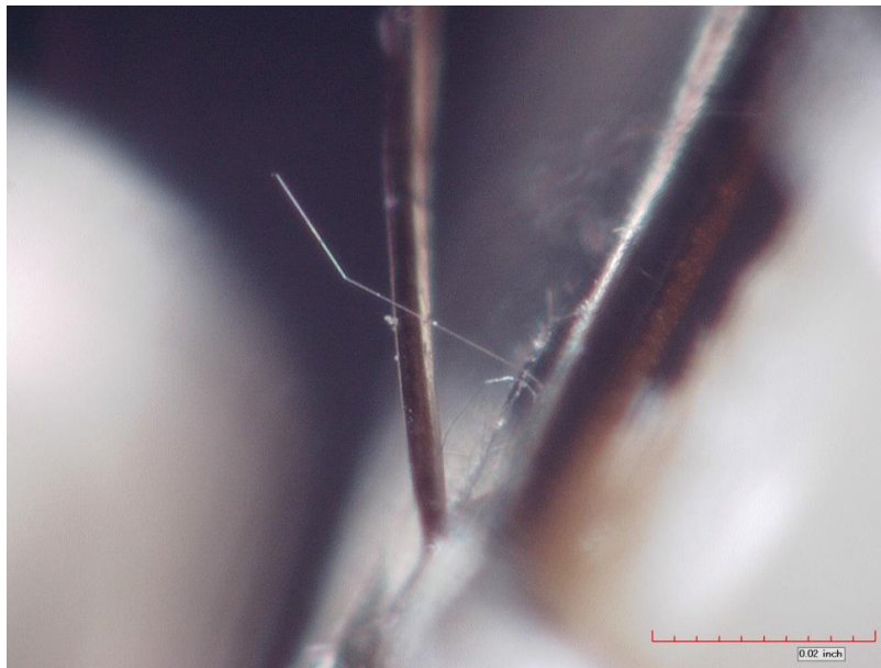
Optical comparison of Human Hair vs. Tin Whisker
