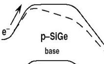
$$\left. \frac{\beta_{SiGe}}{\beta_{si}} \right|_{V_{BE}} \equiv \Xi = \left\{ \frac{\widetilde{\gamma} \, \widetilde{\eta} \, \Delta E_{g,Ge}(grade) / kT \, e^{\Delta E_{g,Ge}(0)/kT}}{1 - e^{-\Delta E_{g,Ge}(grade)/kT}} \right\}$$
