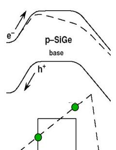
$$\left. \frac{\beta_{SiGe}}{\beta_{si}} \right|_{V_{BE}} \equiv \Xi = \left\{ \frac{\widetilde{\gamma} \, \widetilde{\eta} \, \Delta E_{g,Ge}(grade) / \underline{kT} \, e^{\Delta E_{g,Ge}(0) / \underline{kT}}}{1 - e^{-\Delta E_{g,Ge}(grade) / \underline{kT}}} \right\}$$
