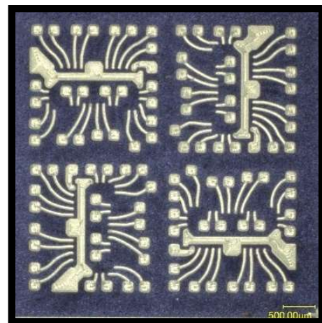
Photo of printed RDL Top (~ 30 µm line width)
