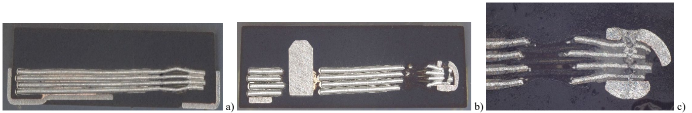
Fig.B.4.2. Overall optical views of cross-sections along terminals (a, b) and close-up of the anode welding (c).
