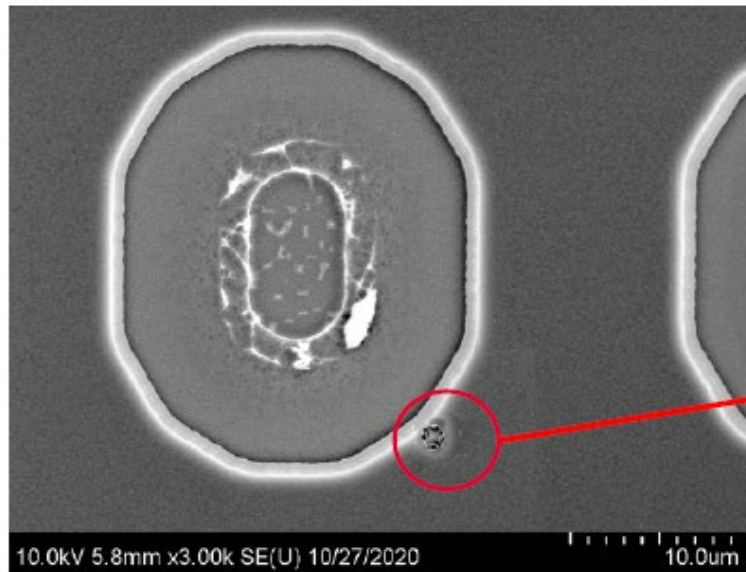
ESD damage on surface and cross-sectioned
