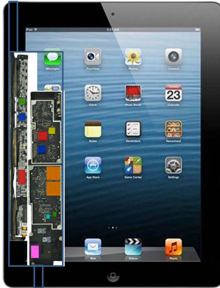
Figure 5.1-6. Approximate position of communications and display boards.
