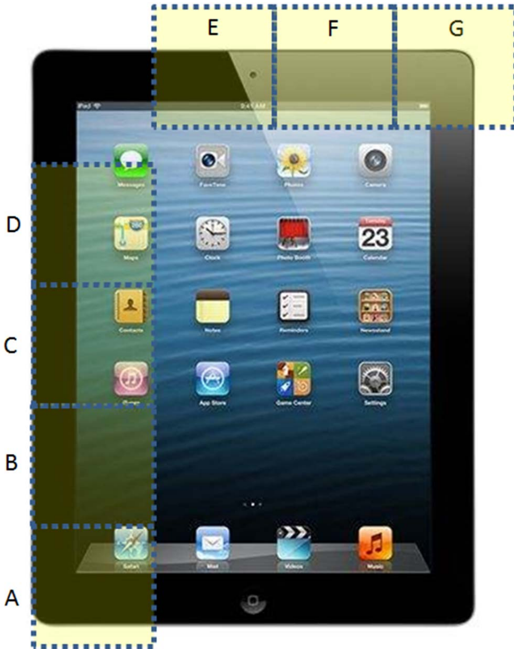
Figure 5.1-7. Beam positions used for proton exposure. The 2-inch (5-cm) square collimator was used for most exposures, and the locations reflect the beam spot size. In addition, positions A–D were alternately exposed with a 1-inch by 2-inch (2.5- × 5-cm) collimator designed to avoid exposure of the display board and battery pack.
