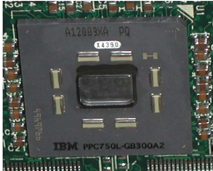
Fig. 3 An example of an advanced microprocessor with an inverted package where the back of the die has been mechanically thinned, leaving approximately 25% of the original die thickness.
