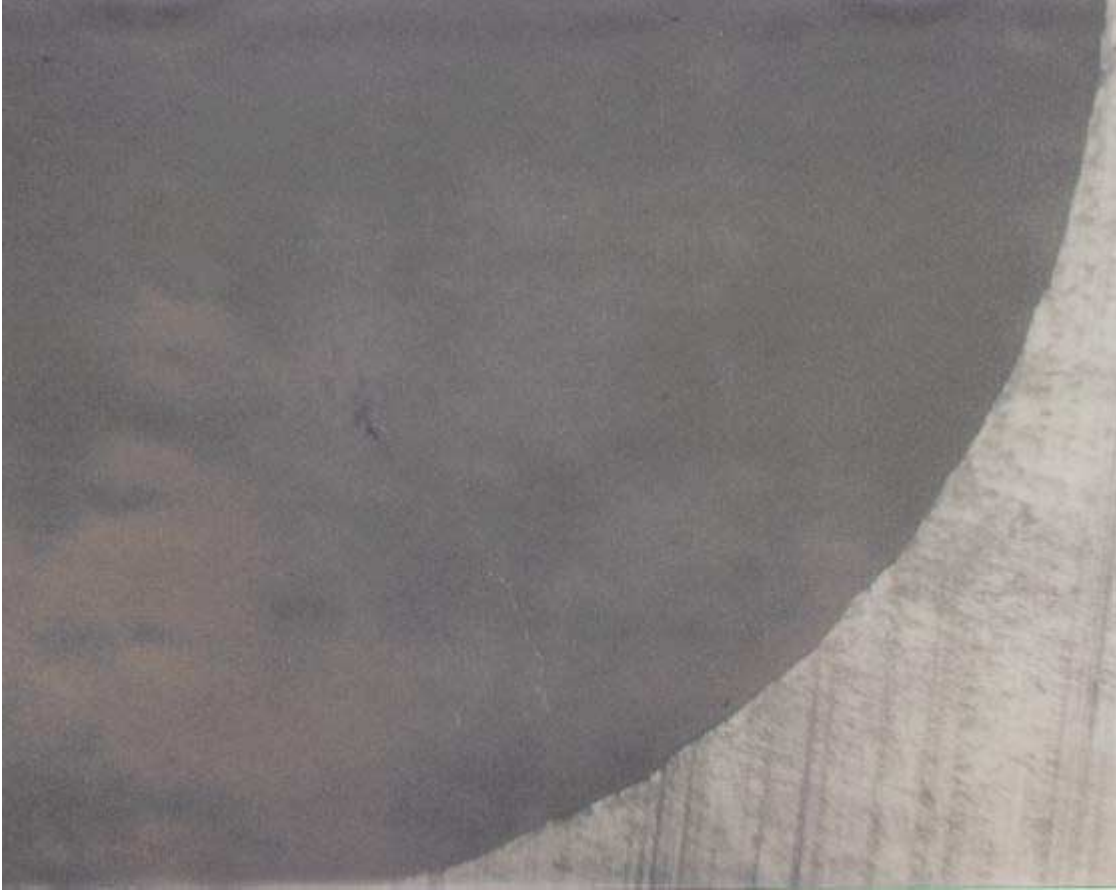
Close Up of an RIE Plasma Etched Via Hole – Large Via – 0.065”
