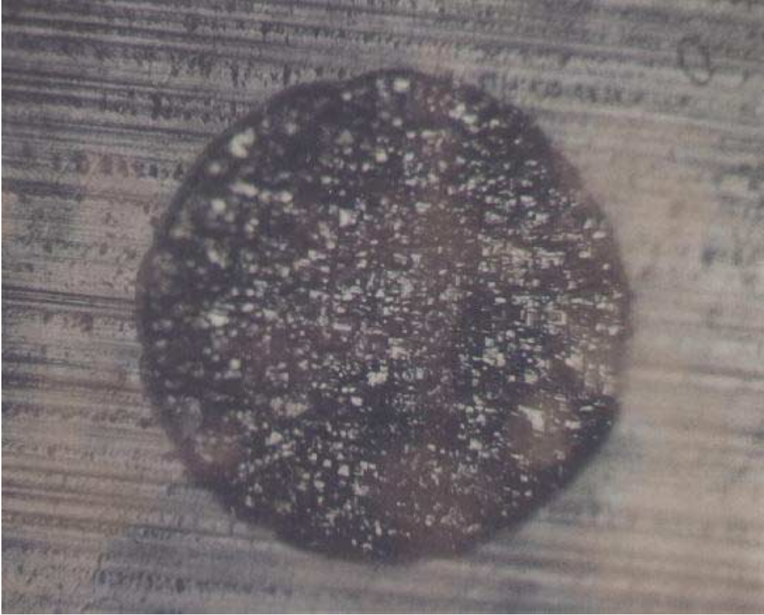
Chemically Etched Via Formed Holes in Aluminum Mask
