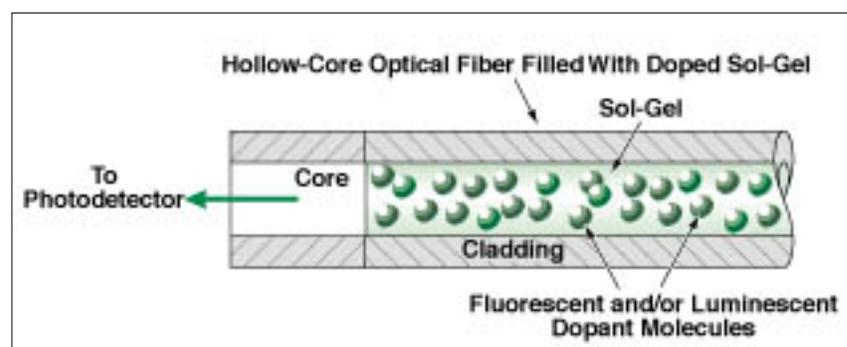
A **Monolithic Core** of sol-gel material with dopant molecules in its pores is formed in an initially hollow optical fiber.
