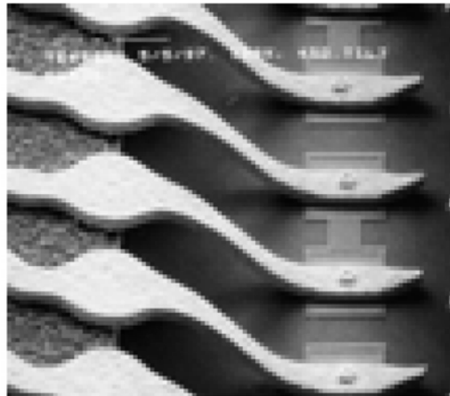
Figure 45. Lead Bonds from Flex Substrate Through Lead Bond Window to Die Pads. [ Solberg-3.pdf ]
