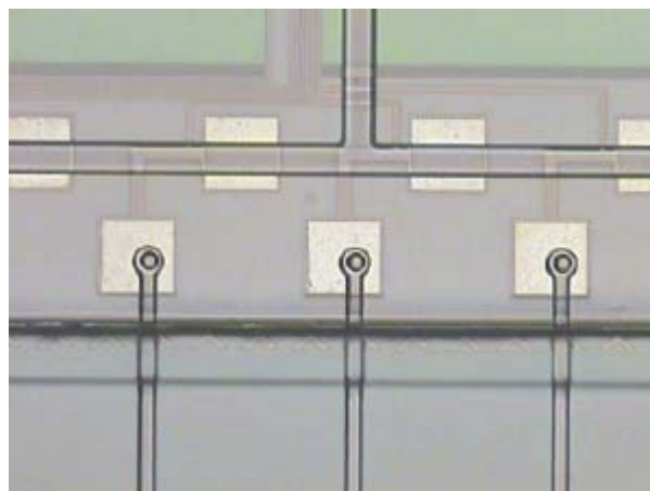
Figure 75. Photograph of thin Film Interconnect to a 15 \mu m Thick Silicon Die. [ Cazaux.pdf ]
