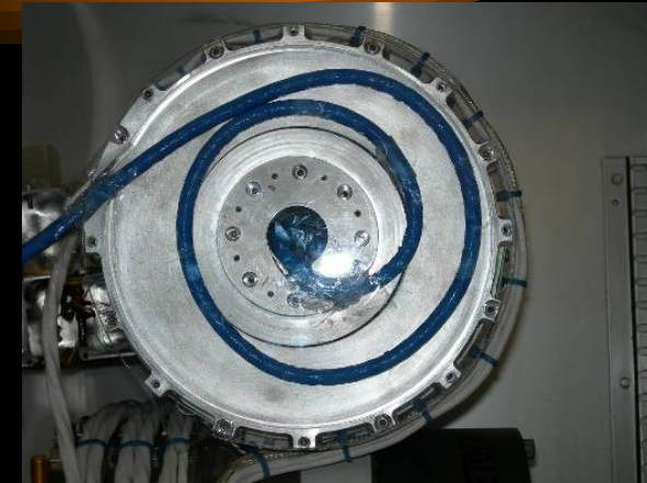
Window inside gimbal; Bundle cable inside.
