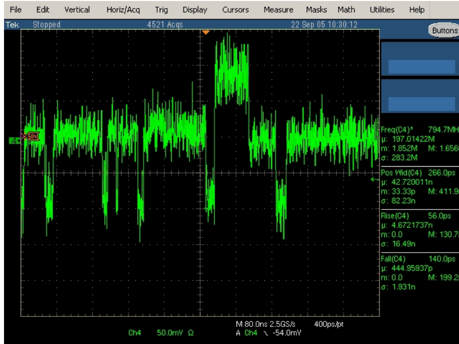
Fig. 2.4.4 Pulses following irradiation with Co-60 gammas to 5 krad(Si). The same operational conditions were used as in Fig.'s 2.4.1 and 2.4.2.
