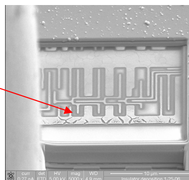
Figure 7. SEM of the defective Region milled with the FIB instrument.
