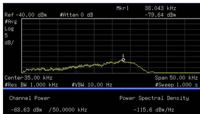
(b) V_{in} = 28.0V , I_{out} = 5.0A , Channel Power Freq. = 38 kHz
