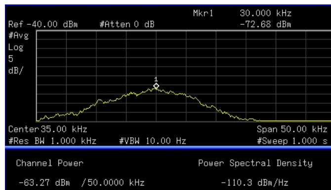
(c) V_{in} = 21.9V , I_{out} = 3.0A , Channel Power Freq. = 30 kHz
