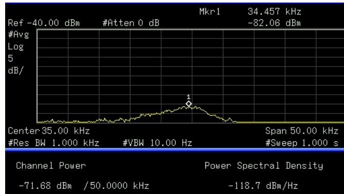
(a) V_{in} = 24.3V , I_{out} = 3.0A , Channel Power Freq. = 34 kHz
