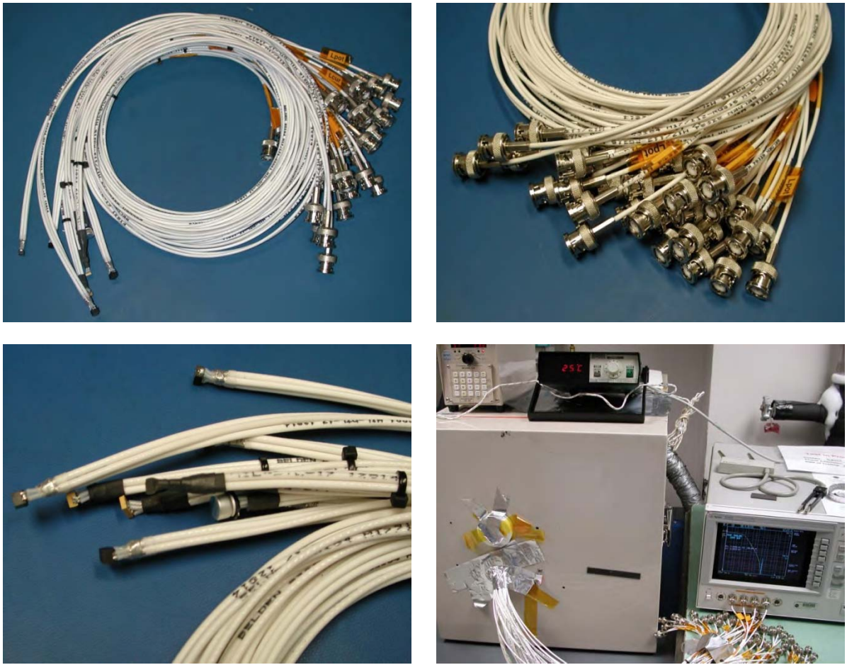
Figure 26. RF cable assembly and the testing set up for the characterization of PA capacitors at a range of temperatures.
