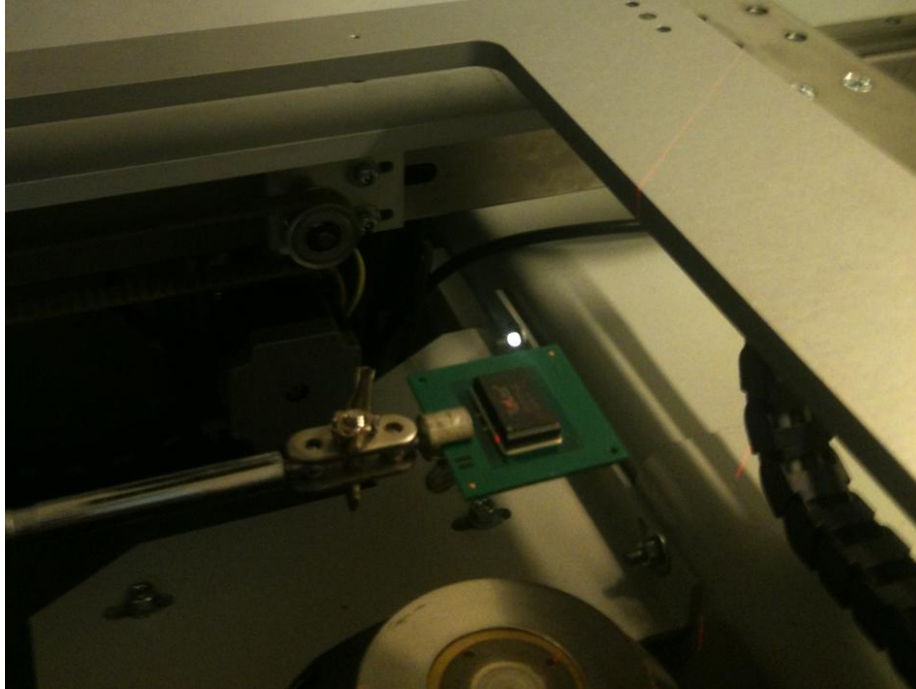
Figure 4.3-1. Photograph of 4-high stack assembly in position and ready for rotation, to generate 3D X-ray images.
