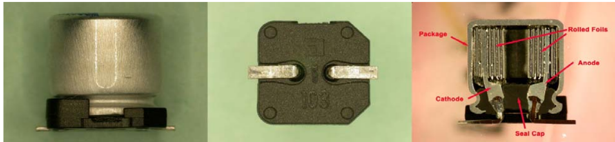
Figure 5. External and cross-section optical views of a 100 µF, 10V PA capacitor made by manufacturer C.
